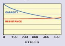
Resistance does not provide a reliable indication on capacity fade that occurs with cycling.  $QuickSort^{TM}$  is based on the electrochemical dynamic response of the battery, a method that is superior to resistance readings.
